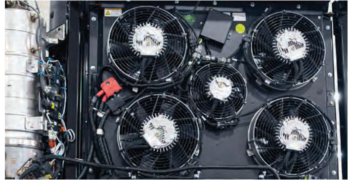
Remote mounted 1,814 square inch radiator produces quieter, cooler cab environment and allows for a pass through cab design
