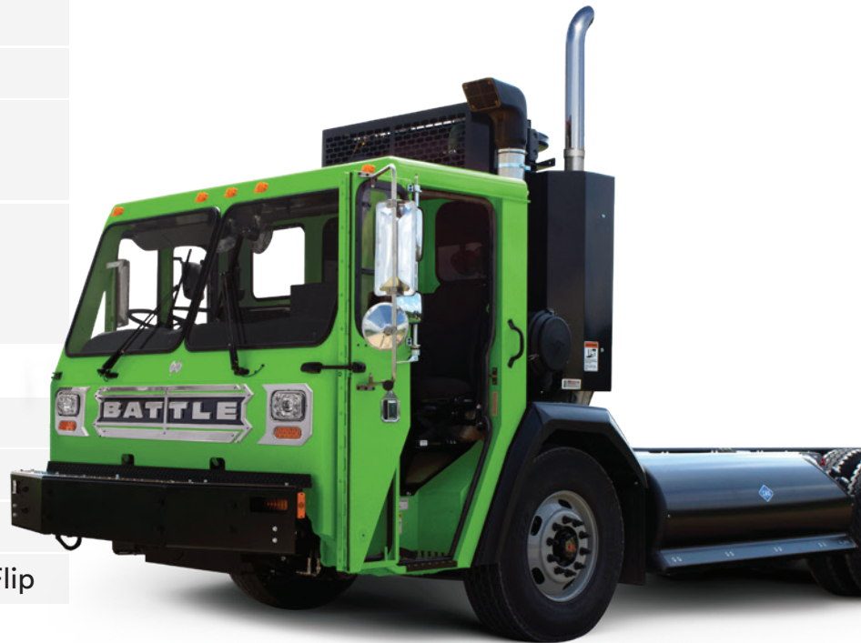
Fuel Management Module (FMM) integrated into all BTC and saddle mount systems NGV-1 and Transit Quick Connect Fuel Fill Connections located in FMM Factory installed, warranted, and supported CNG systems in both BTC and saddle mount configurations from 45 DGE to 75 DGE
