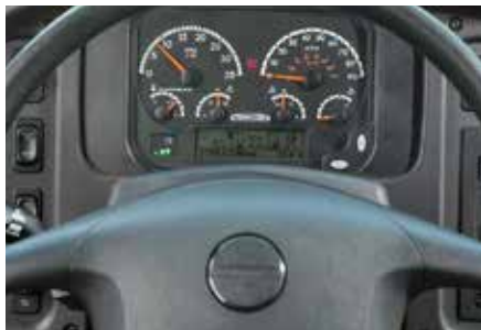
A non-reflective instrument panel features easy-to-read, LED-backlit gauges
