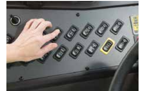
A multiplex-wired Smart Switch system offers easy access to switches and is designed to meet drivers' preferences without re-wiring
