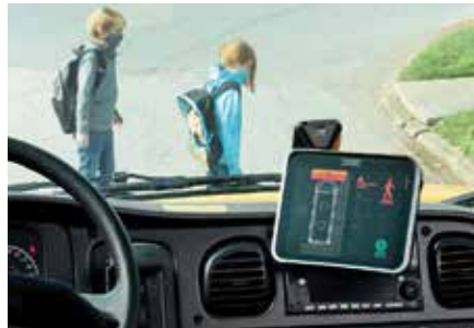
Saf-T-Zone Pedestrian Detection alerts warn drivers via tablet when pedestrians enter the danger zone
